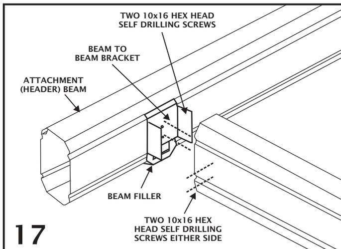
If any intermediate columns are required measure the valley beam marking where they meet. Fasten post brackets as explained in the Stratco Installation Guide: 'Pergola Flat Attached Verandah, Patios & Carports' under "Bracket and Filler Connections". This can be done before valley beams are fixed in place.
