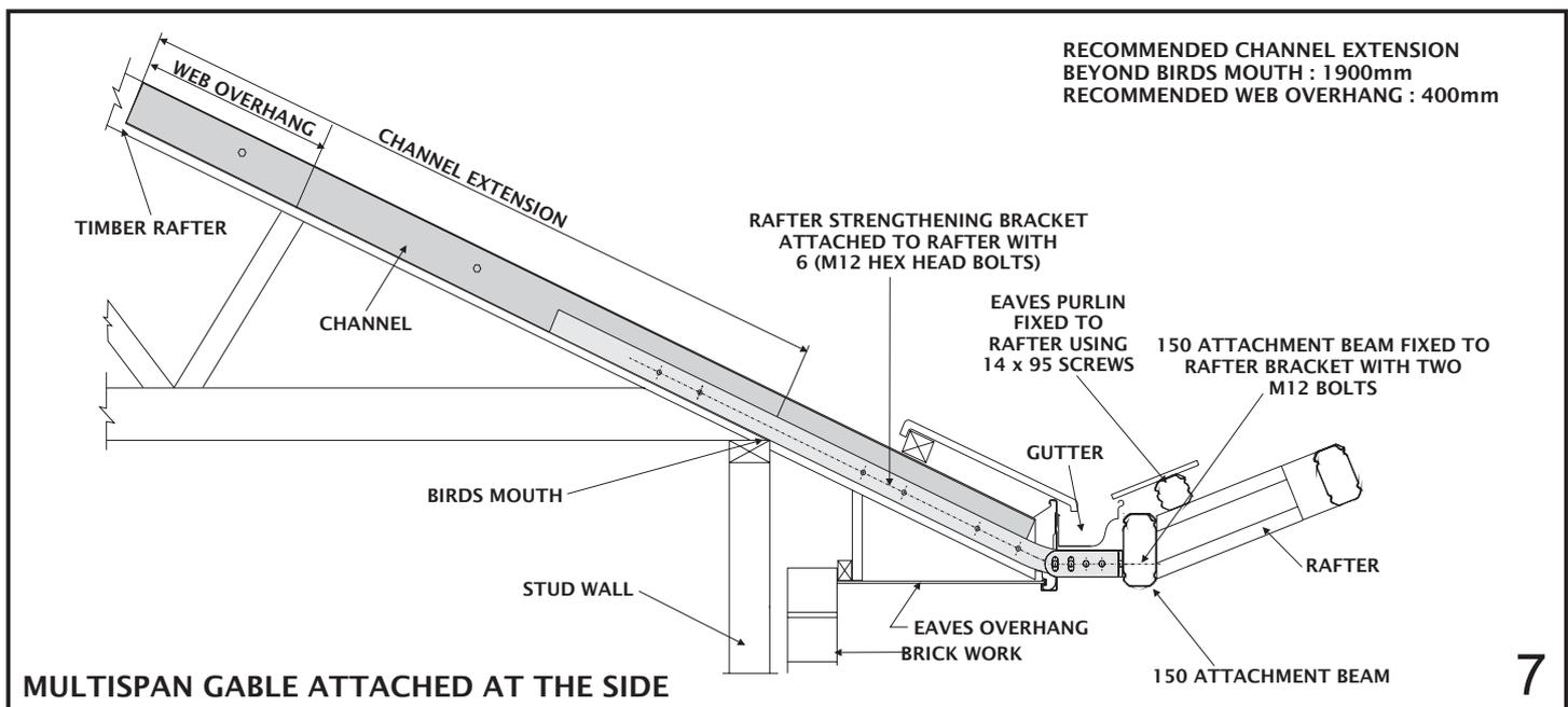
The 150 attachment beam becomes the base for the attachment of the Multispan gable unit. Figure 7 shows a unit attached at the side.
