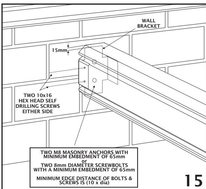
For units attached on the end to a fascia, suspension brackets are positioned at either side of the gable opening at the spacing determined in Section 3.0 (Figure 13).
