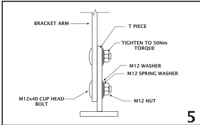
Insert the bracket through the fascia and fix with the channel to the house rafter using M12 hex head bolts through the existing holes in the bracket and further up the channel (Figure 7). Adjust the T piece so it is horizontal and has the appropriate extension past the fascia to allow for fixing of the attachment beam. T piece connection bolts are to be tightened to a minimum 50Nm torque.
