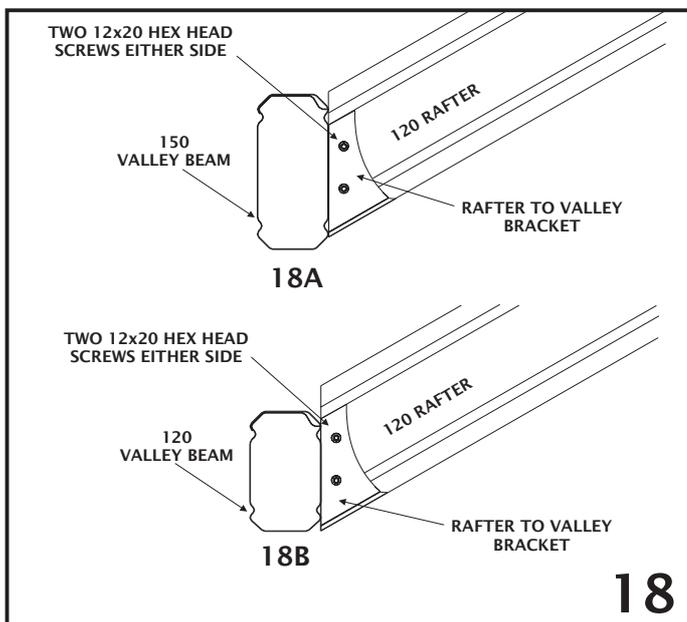
Fix the gable rafters into the rafter to valley brackets with two 12x 20 hex head screws either side (Figure 18).
