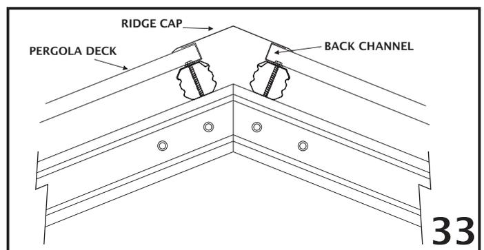
For polycarbonate and corrugated roofing screw or rivet (depending on ridge cap style) the ridge cap directly onto the top of the deck. Waterproof rivets with silicone.
